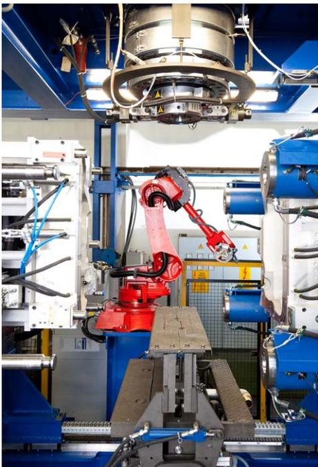
Clamping unit with ring insert robot
